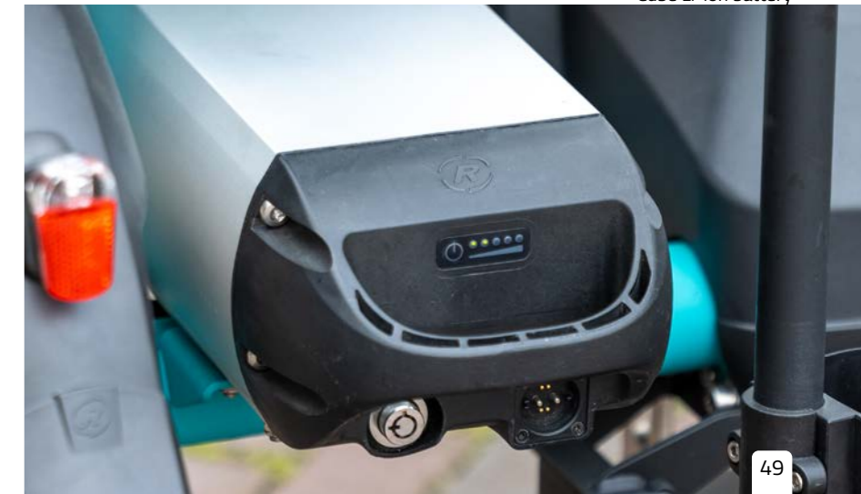
Cube Li-ion battery
